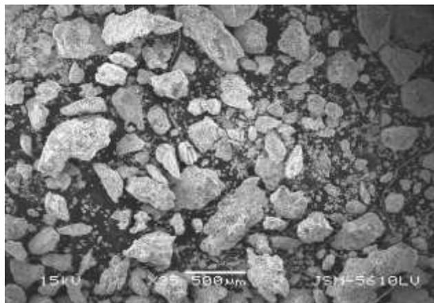
Figure 2 SEM image of  $\text{Bi}_2\text{S}_3$  with capping agent CTAB
