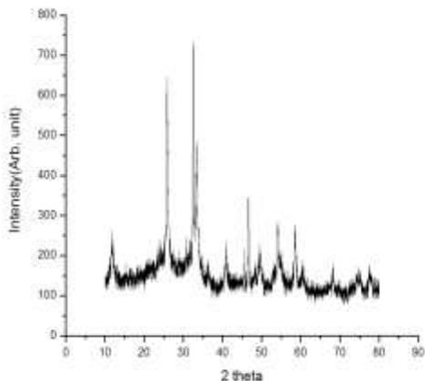
Graph 1- X-ray diffraction pattern of  $\text{Bi}_2\text{S}_3$
