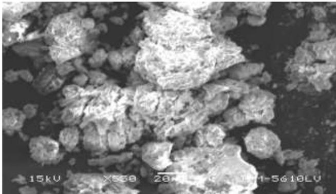
Figure 4 SEM image of  $\text{Bi}_2\text{S}_3$  with capping agent CTAB
