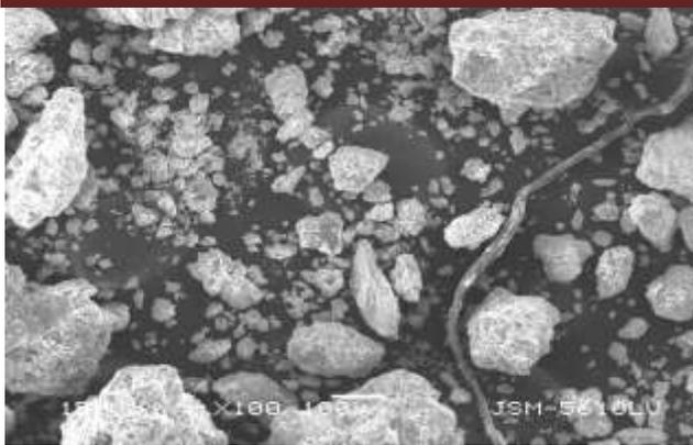
Figure 3 SEM image of  $\text{Bi}_2\text{S}_3$  with capping agent CTAB
