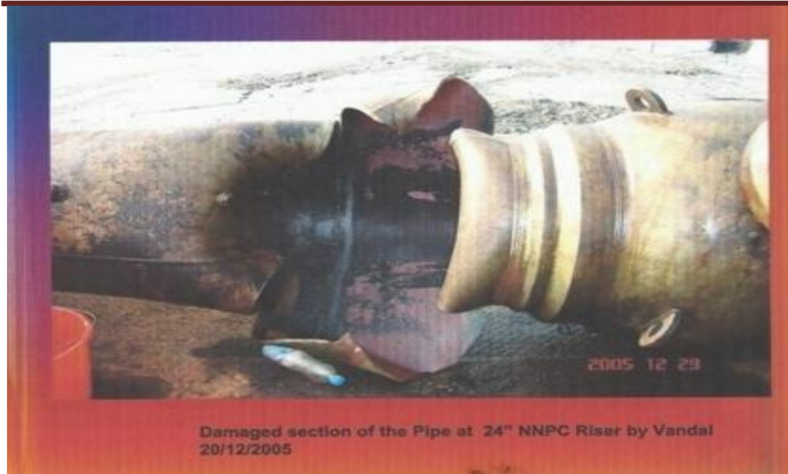
Plate 4: Showing a damaged oil pipeline, as a Result of Illegal Bunkery Activities.
