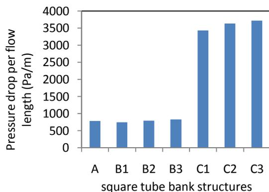
Figure 6: Pressure drop per flow length unit in different arrangements for Reynolds 40000
