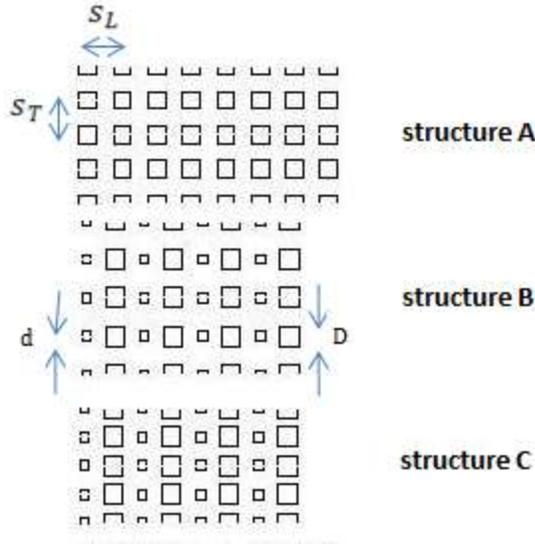
Figure 1: Geometry of the problem and the different structures of a square tube bank
