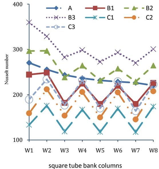
Figure 4: Distribution of the flow Nusselt number according to the square tube bank columns with different arrangements for Reynolds 40000
