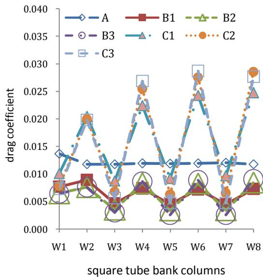
Figure 5: Distribution of the flow drag coefficient according to the square tube bank columns with different arrangements for Reynolds 40000
