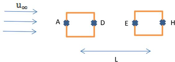
Figure 2: Schematic view of two square cylinders and measured points of the pressure coefficient
