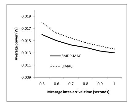
Figure 3: Average power consumption, linear topology
