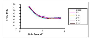
Fig.3 Comparison of BSFC v/s Brake power
