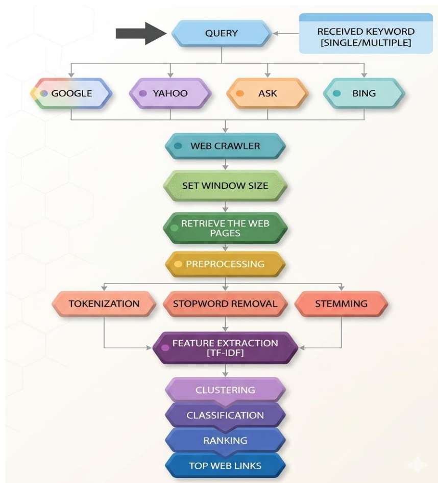
FIG. 6: ARCHITECTURE FOR TEXT MINING BASED SEARCH ENGINE
