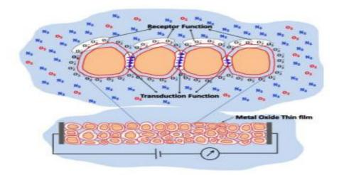
Figure 1 Schematic of metal oxide thin film gas sensor
