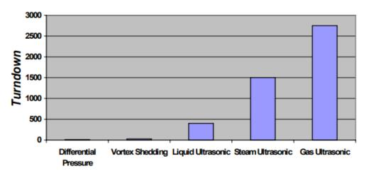
Figure 1: Turndown Ratio of Some Common Flow meter Types, Including Transit Time Ultrasonic Flow meter
