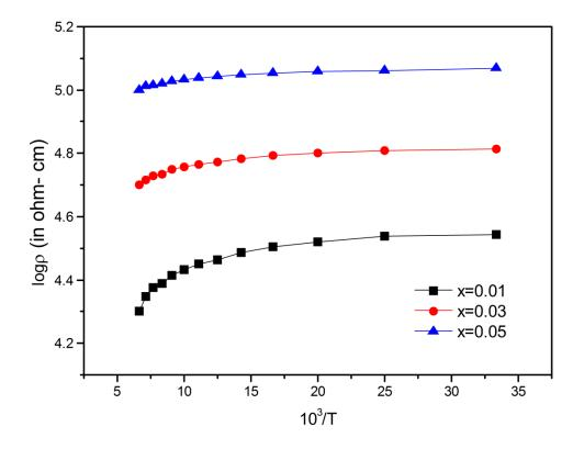
Figure 2: Variations of log  $\rho$  with 1000/T in Mg<sub>x</sub>Mn<sub>1-x</sub>Fe<sub>2</sub>O<sub>4</sub> ( x= 0.01, 0.03, 0.05) ferrites
