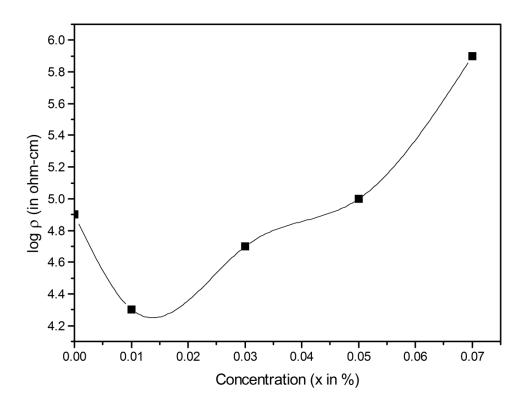
Figure 1. Variations of log  $\rho$  with concentration of  $Mg^{2+}$  ions in  $Mg_xMn_{1-x}Fe_2O_4$  ferrites at  $150^oC$
